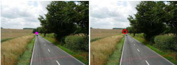
(c) Vanishing point estimation: the left image using the Kong's algorithm, the right image using the proposed algorithm
